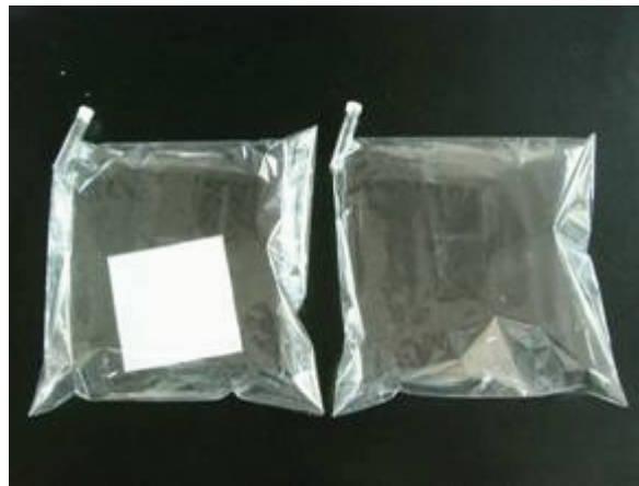
Figure 2 — After injection of quasi unpleasant odour gas in plastic bags with or without specimen
