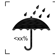
Figure 4 — Maximum humidity of storage conditions
