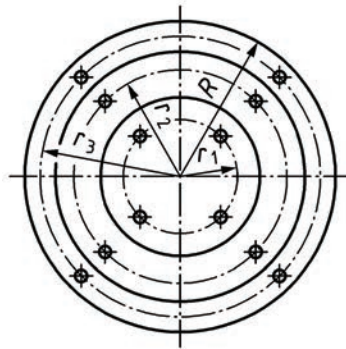
Figure 2 — Air velocity measuring points of round duct
