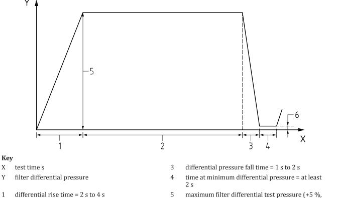
Figure 1 — Differential pressure waveform for cold start test
