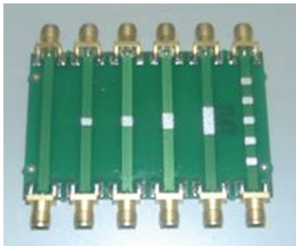
Figure 8 — Assembly of standard test circuit board for measurement in the X-Y plane
