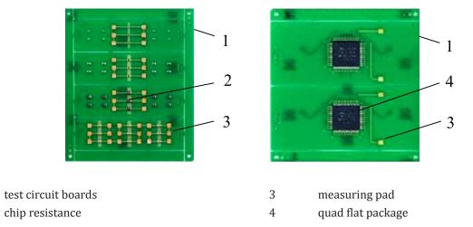
Figure 2 — Example of the position of components
