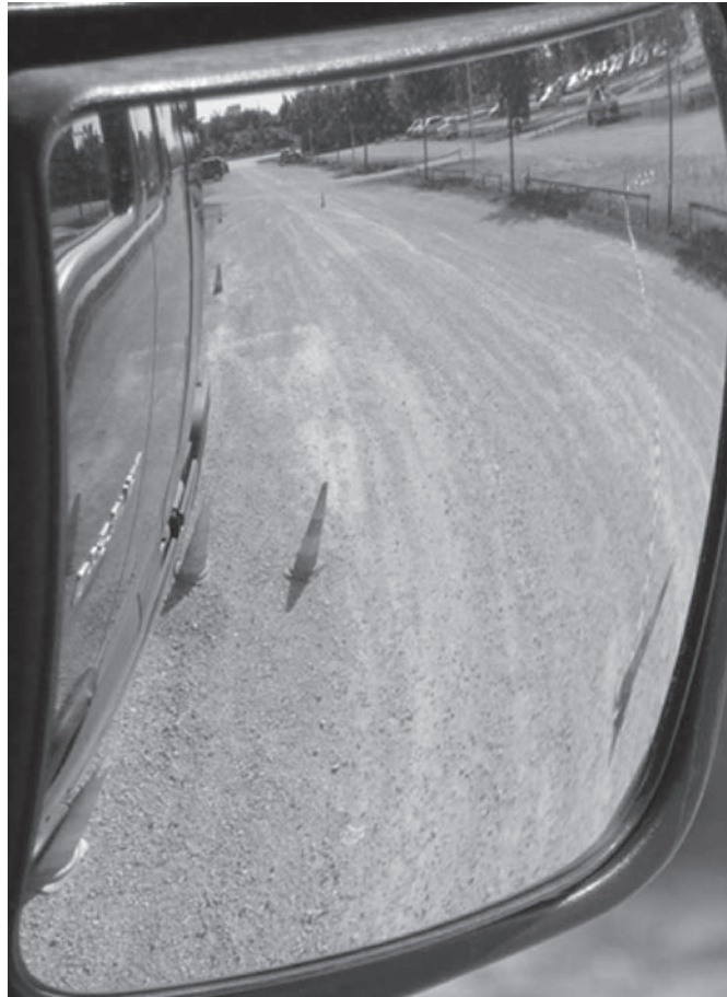
Figure B.19 — Magnification factor variation exemplified with a class IV mirror field of view
