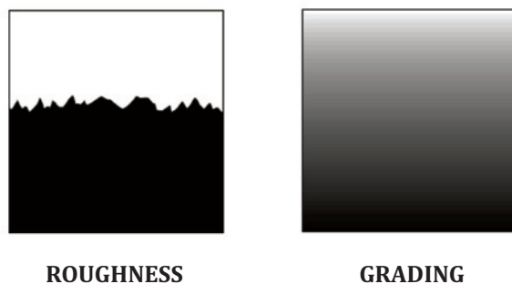
Figure 6 — Roughness and grading of a surface
