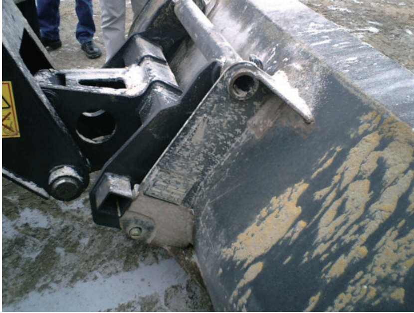
Figure 9 — User-added welds shown in photo
