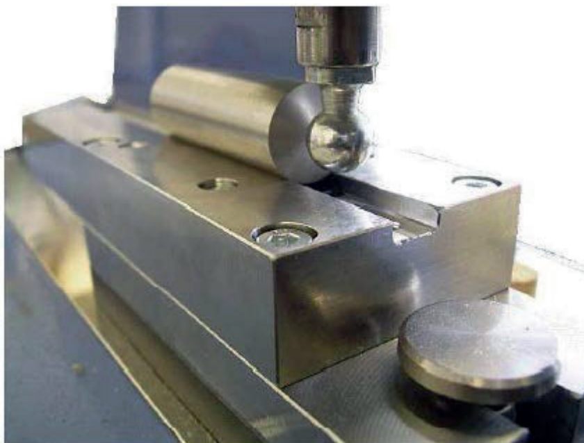
Figure C.3 — Mounted impact device with a cylindrical mass piece and pendulum bob
