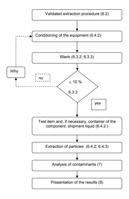
Figure C.1 — Synopsis of the test procedure
