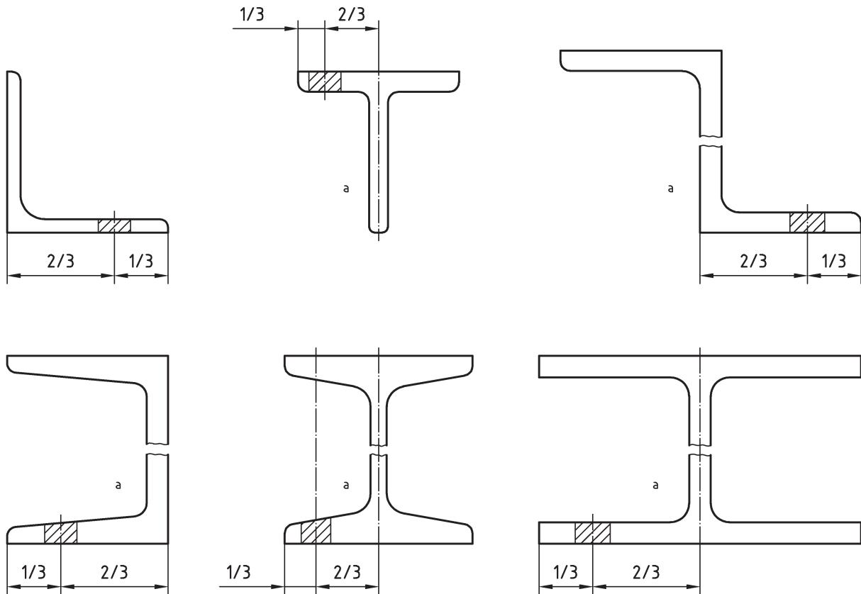
**Figure 3 — Position of test pieces (hatched) for beams, channels, angles, T sections, and Z sections**
