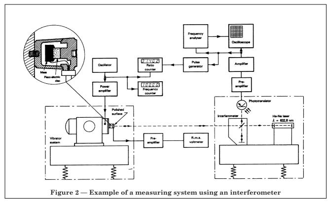
The object of the reciprocity method is to determine the sensitivity  $S_{\rm uc}$  that when the potential difference  $u_{13}$  is measured, the acceleration  $\hat{a}$  may be computed by use of equation (8).  $S_{\rm uc}$  is determined from the following equation:
