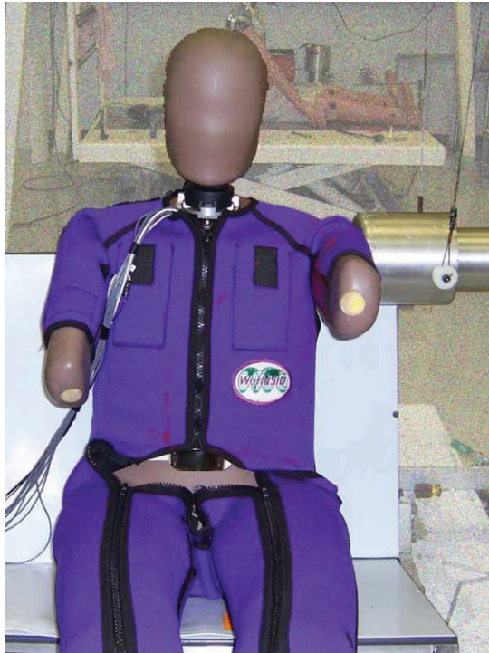
Figure 9 — Shoulder test, dummy and arm position
