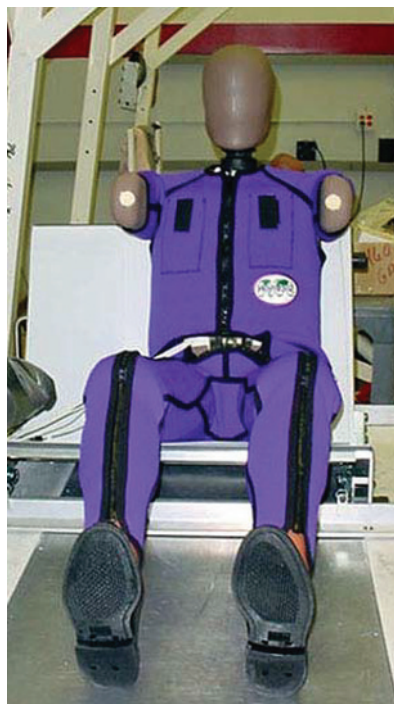
Figure 6 — Front view of setup for full dummy validation tests
