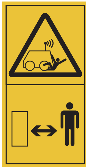
Figure A.1 — Example of machine safety label
