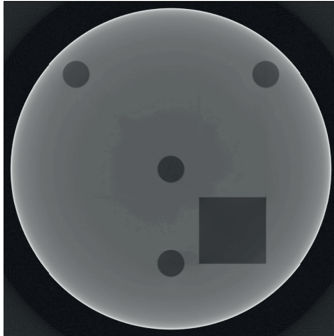
Figure 6 — Example of cupping effect[2]
