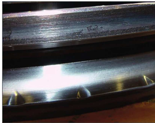
Figure 26 — Overload on a stationary inner ring of an angular contact ball bearing
