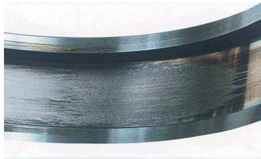
Figure 11 — Smearing on the outer ring raceway of a cylindrical roller bearing
