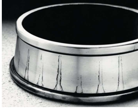
Figure 16 — Contact corrosion at roller pitch on the inner ring raceway of a tapered roller bearing
