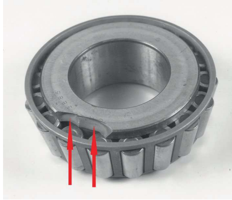
Figure 33 — Forced fracture of a tapered roller bearing inner ring shoulder, caused by an impact load during assembly procedures
