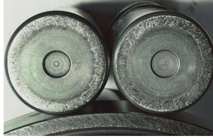
Figure 13 — Smearing on the side face of rollers of a cylindrical roller bearing
