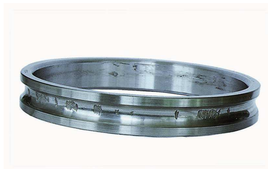
Figure 27 — Spalling as a result of shock load deformation on the inner ring raceway of an angular contact ball bearing, resulting from impacts in radial direction, which further developed in spalling
