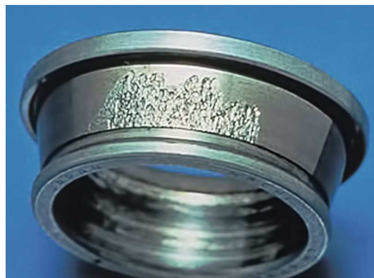
Figure 4 — Advanced subsurface spalling in a tapered roller bearing — Stationary inner ring
