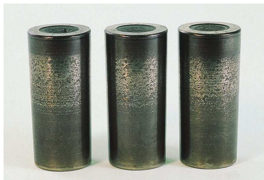
Figure 31 — Indentations from particles on tapered rollers
