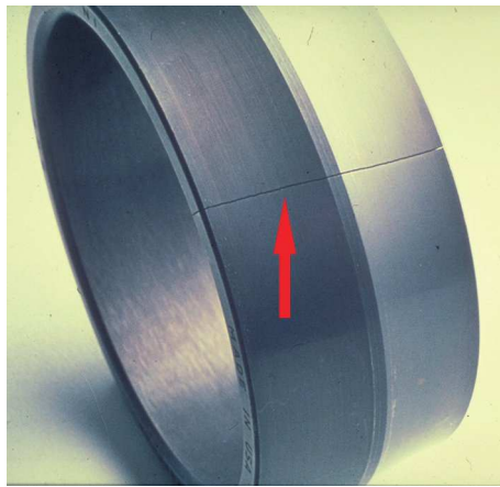
Figure 33 — Forced fracture of a tapered roller bearing inner ring shoulder, caused by an impact load during assembly procedures
