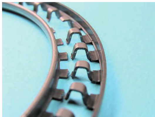
Figure 36 — Fatigue fracture of cage bars of a needle roller thrust bearing
