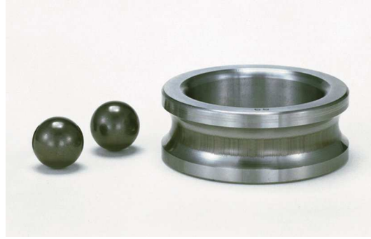
Figure 24 — Fluting on the inner ring raceway and matt dark grey coloured balls of a deep groove ball bearing
