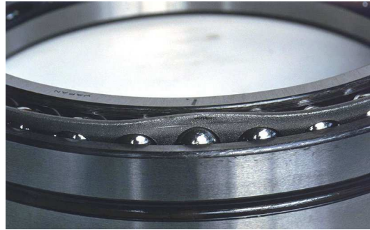
Figure 28 — Cage deformation of an angular contact ball bearing caused by a shock load during handling
