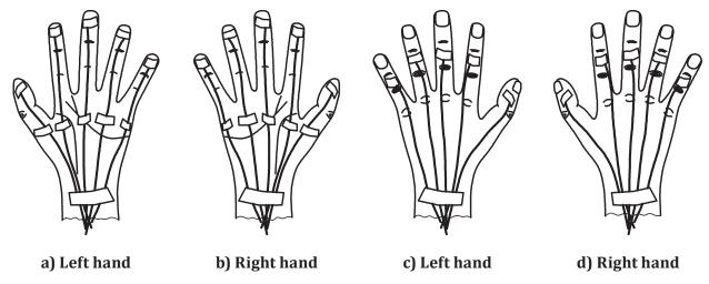
NOTE Attachment of sensors on the fingertips is recommended [see a) and b)]. An optional method of attachment on the dorsal surfaces of the distal (thumb) or middle phalanges is also shown [see c) and d)].
