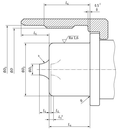
Surface roughness values in micrometres and in accordance with ISO 1302
