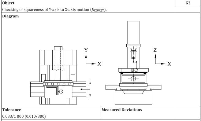
Straightness reference artefact, squareness reference artefact and linear displacement sensor, or optical measuring instruments
