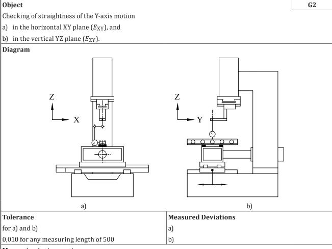
Straightness reference artefact and linear displacement sensor, or optical measuring instruments
