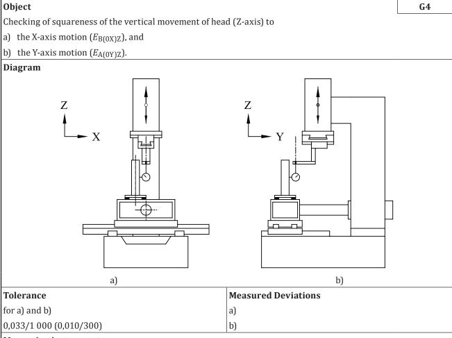
Squareness reference artefact, surface plate, adjustable blocks and linear displacement sensor, or optical measuring instruments
