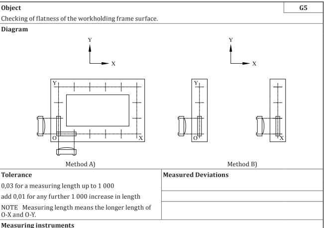
Method A) Precision level, or optical measuring instruments
