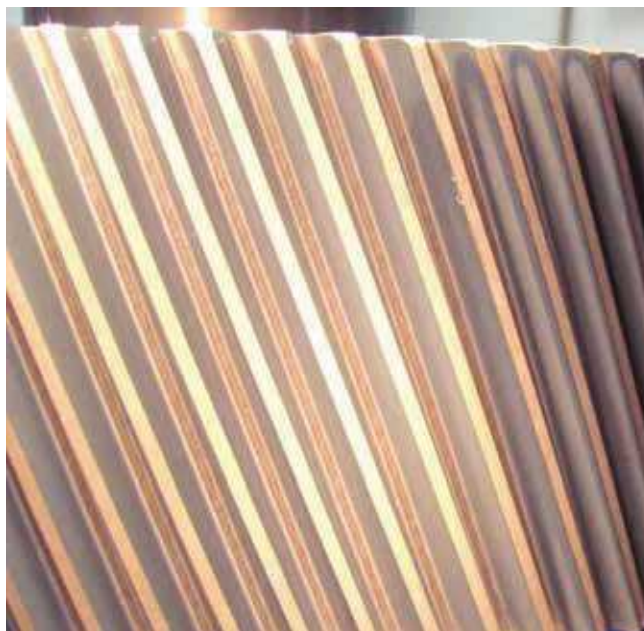
Figure 6 — Progressively worse surface temper of teeth from left with Class FA no tempering to right with Class FE rehardening surrounded by Class FD heavy tempering on four teeth at right
