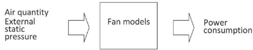
Figure D.15 — Inputs and outputs of fan models
