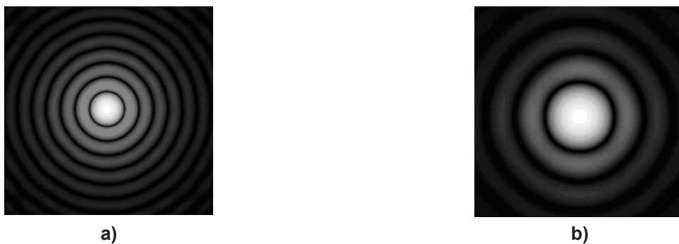
Figure 1 — Scattering pattern for two spherical particles: the particle generating pattern a) is twice as large as the one generating pattern b) (simulated images for clarity)
