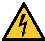
Figure 1 — Symbol of voltage class B electric components
