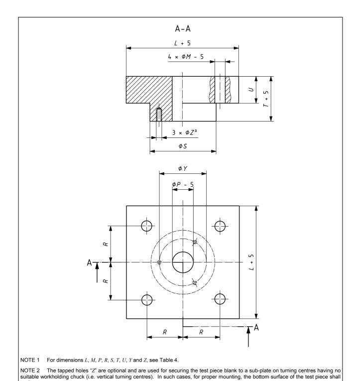
Figure 1 — Test M3 pre-machined blank
