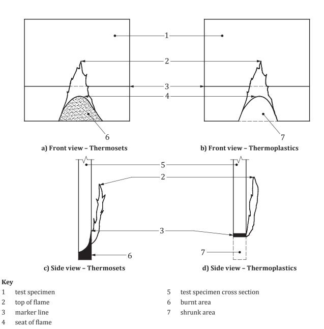
Figure 1 — Identification of seat of flame
