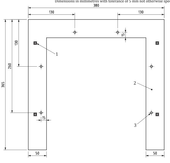
Dimensions in millimetres with tolerance of 5 mm not otherwise specified  $\,$
