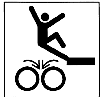
A.4.5 Falling into machinery — Rollers
