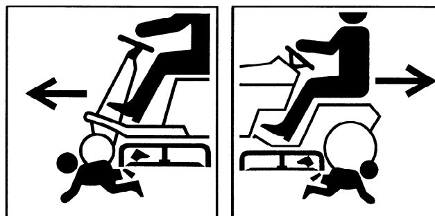
Figure D.23 — Examples of pictorials using arrows to represent direction of motion of entire machines
