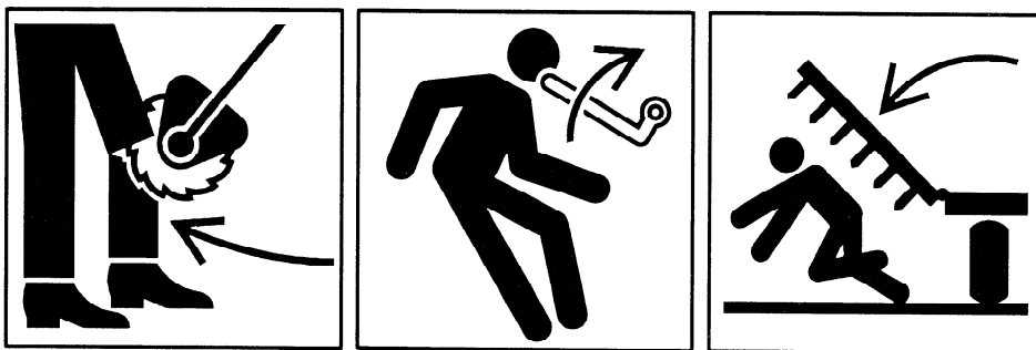
Figure D.21 — Examples of pictorials using arrows to represent direction of motion of machine components
