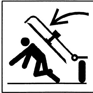
A.6.15 Crushing — Rotary cutter
