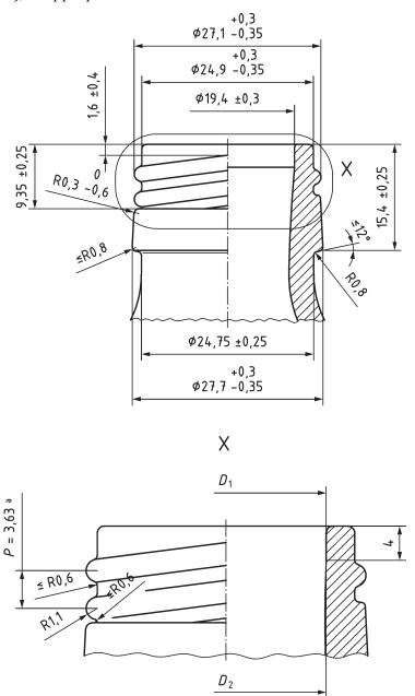
NOTE Diameter  $d_2$  at 4 mm depth and  $\geq \emptyset$  17 mm.
