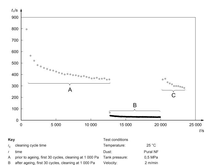
Figure 3 — Development cycle duration versus time before and after ageing
