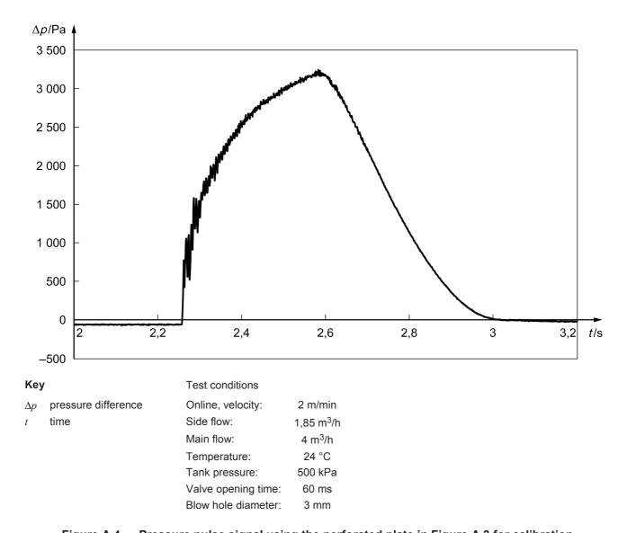
Figure A.4 — Pressure pulse signal using the perforated plate in Figure A.3 for calibration
