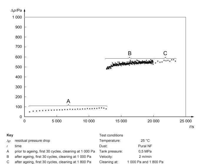
Figure 2 — Development of residual pressure drop versus time before and after ageing
