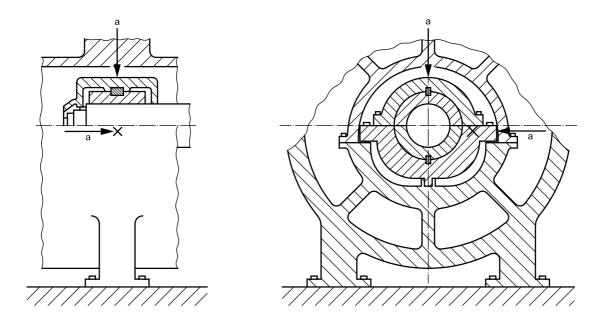
NOTE The evaluation criteria in this part of ISO 10816 are applicable to radial vibration on all main bearings and to axial vibration on thrust bearings.
