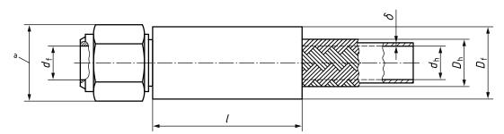
Width across corners of nut and socket hexagon may exceed the values given for  $D_f$  (see footnote b of Table 2).
