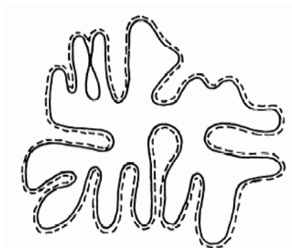
Figure 2 — Schematic cross-section of a particle with surface detected by the adsorption method shown by dotted line
