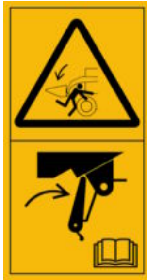
Figure C.10 — Crushing of whole body — Secure locking device before entering hazardous area — Read operator's manual
