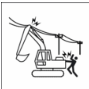
Figure A.5 — Electrical shock/electrocution — Loader
