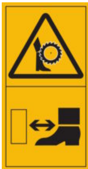
Figure C.22 — Severing of foot or leg — Keep feet and legs safe distance from hazard
