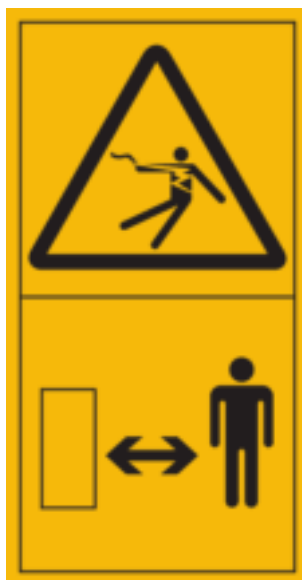
Figure C.14 — Electrical shock or electrocution — Stay safe distance from electrical power source
