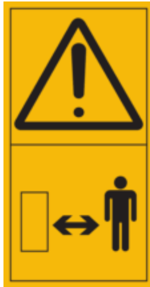
Figure C.1 — Stay safe distance from hazard — General
