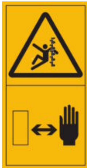
Figure C.25 — Arm or hand entanglement in auger — Keep hands and arms safe distance from hazard
