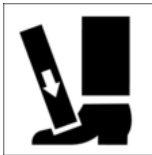
Figure A.19 — Crushing of whole body — Excavator
