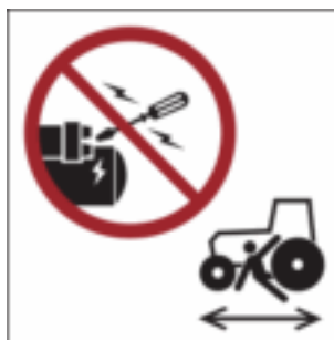
Figure D.26 — Example of pictorial using general prohibition sign to communicate prohibited action
