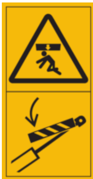
Figure C.7 — Crushing of whole body — Secure lift cylinder with locking device before entering hazardous area
