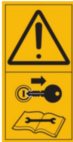
Figure C.12 — General safety alert — Shut off engine and remove key before performing maintenance or repair work
