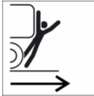
Figure D.21 — Example of pictorial representing direction of motion of entire machines
