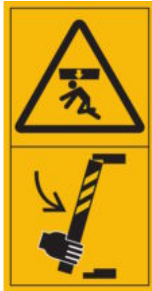
Figure C.8 — Crushing of whole body — Attach support before entering hazardous area
