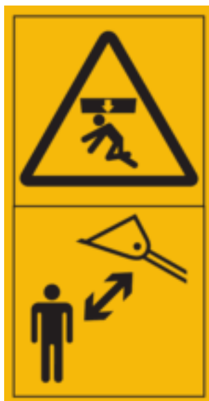
Figure C.30 — Crushing of whole body — Stay safe distance from raised loader lift arm and bucket
