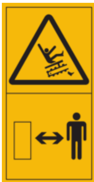
Figure C.27 — Leg or foot entanglement or severing — Stay safe distance from hazard
