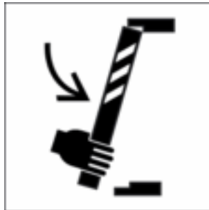
Figure B.8 — Secure lifting cylinder with locking device before entering hazardous area
