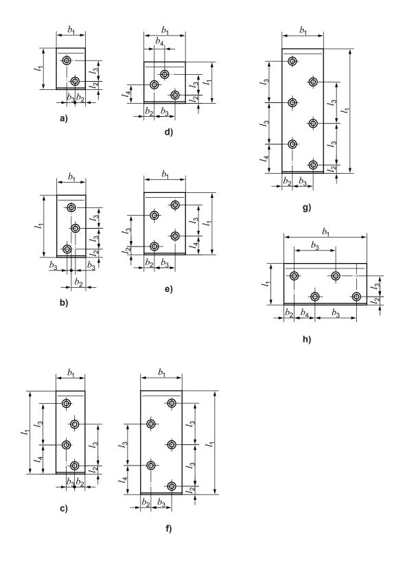
Figure 2 — Clearance hole patterns
