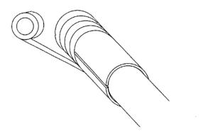
Figure A.3 — Winding tape over the tabs
