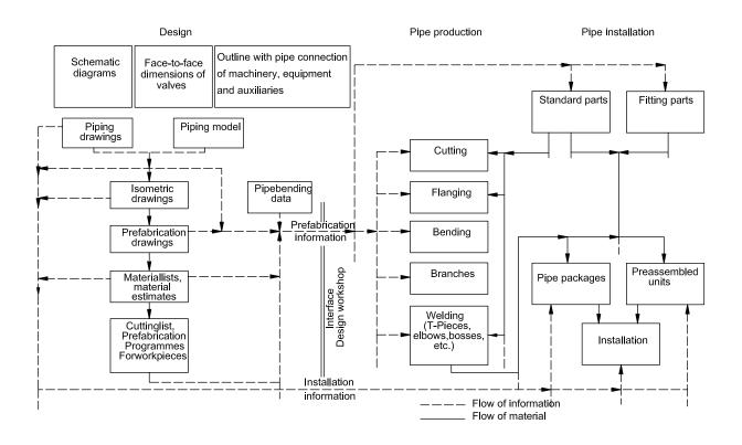
Figure 1 — Data and material flow for pipe production and installation
