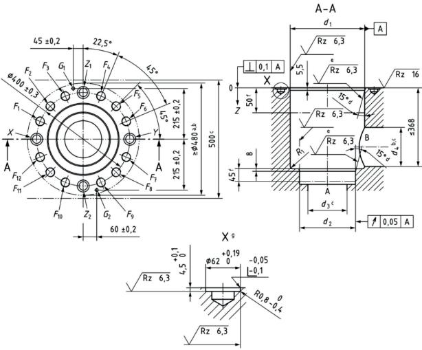
Dimensions and geometrical tolerances in millimetres
