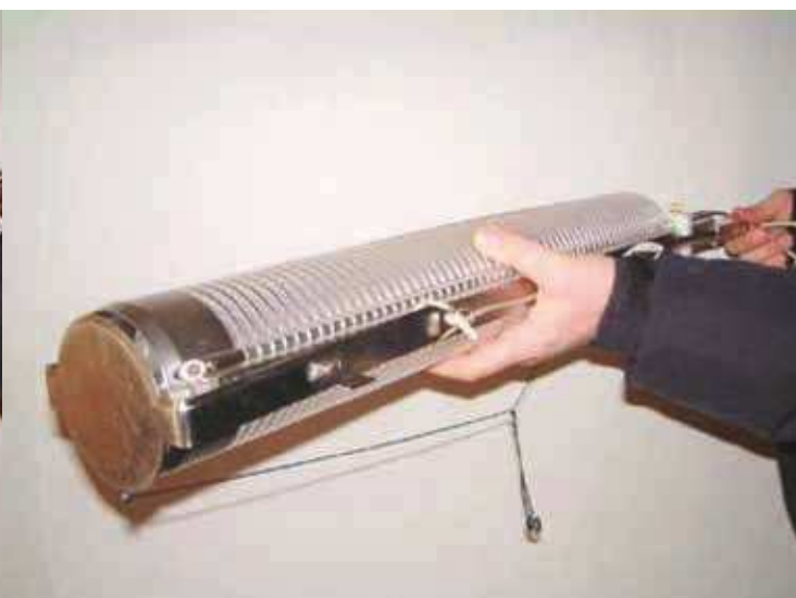
Figure M.1 — Sediment sampler with slicing mechanism
