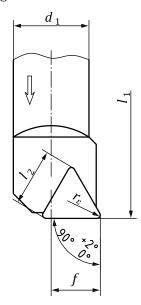
NOTE This figure shows a right-hand tool holder (R); left hand tool holder (L) laterally reversed.
