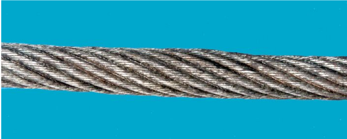
Figure B.16 — Local increase in rope diameter due to core distortion
