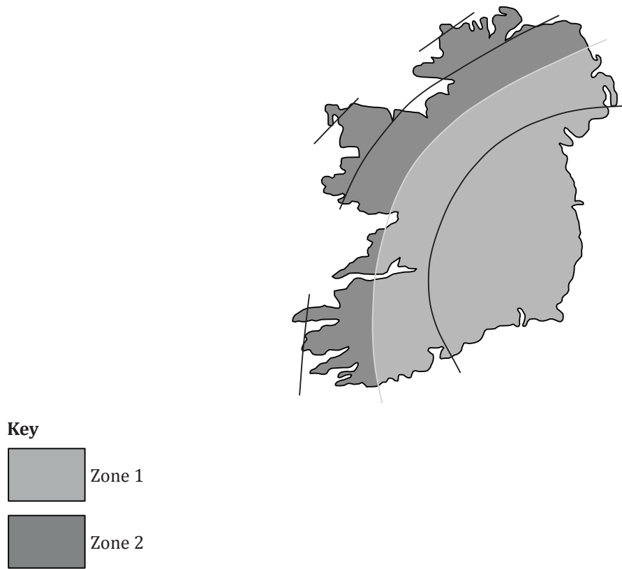
Figure A.3 — Map of Ireland indicating regions where the same reference storm wind speeds are applicable
