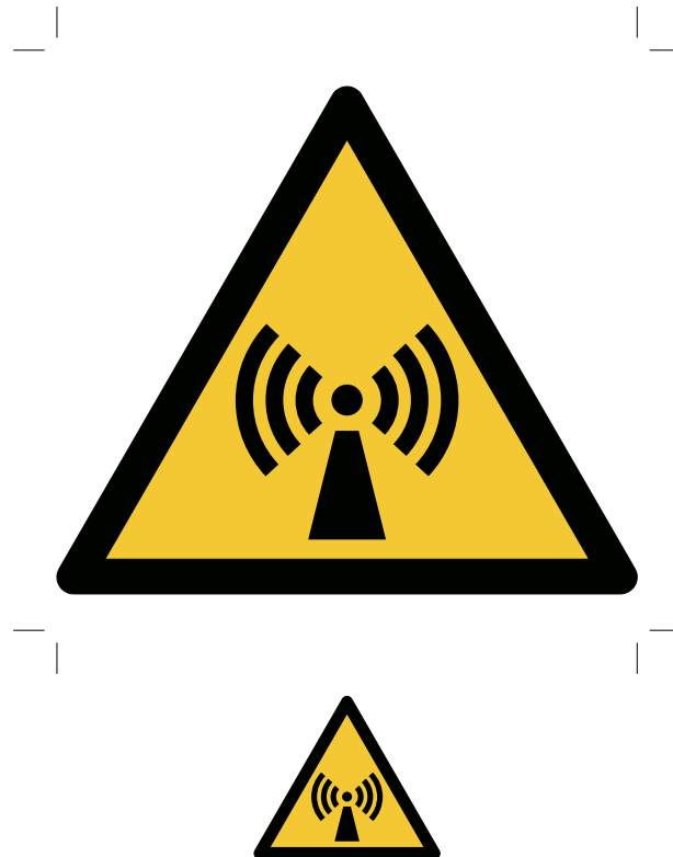
Figure 13 — Warning; Non-ionizing radiation (ISO 7010-W005) — Original size (70 mm) and size reduction to 25 %
