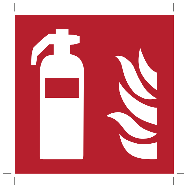
Figure 6 — Fire extinguisher (ISO 7010-F001)
