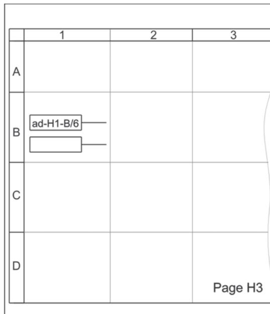
**Figure 2 — Extended jumping reference for continuous lines in a circuit diagram consisting of more than one page**
