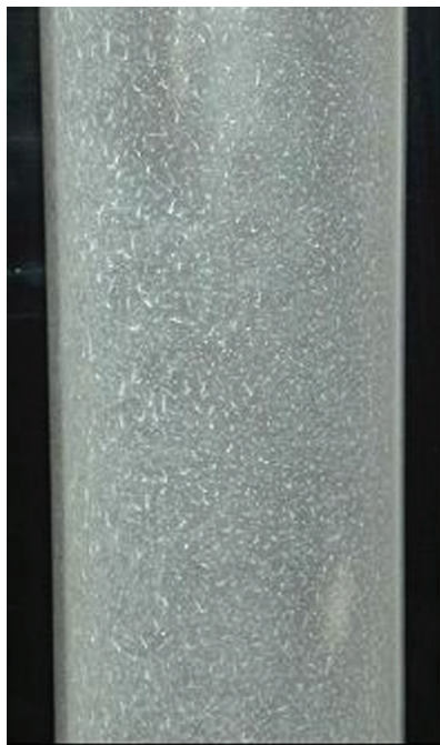
Figure C.5 — Tube etching due to hydrogen fluoride
