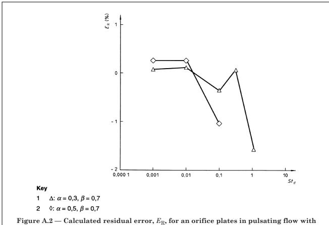
Figure A.2 — Calculated residual error,  $E_{
