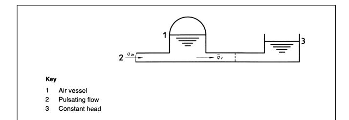
Figure 4 — Use of an air vessel in pulsating liquid flows
