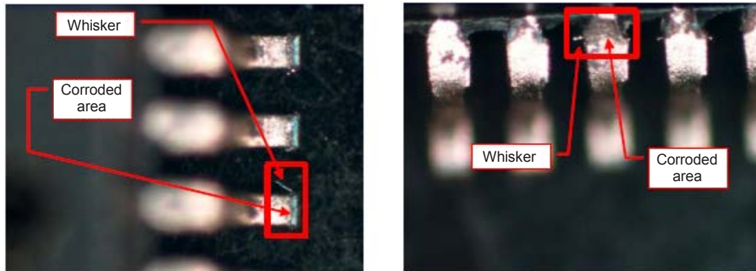
Figure A.3 – Examples of whiskers in areas of corrosion
