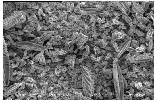
d) Dendrites formed on a tin surface during plating. These are not tin whiskers
