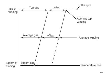
Figure B.1 – Temperature distribution model
