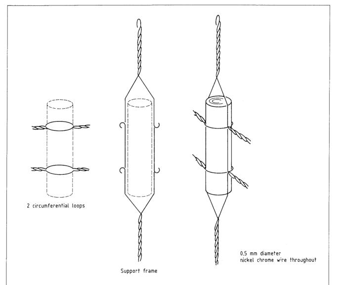
Figure 2. Suggested support method for cylindrical and rectangular cells
