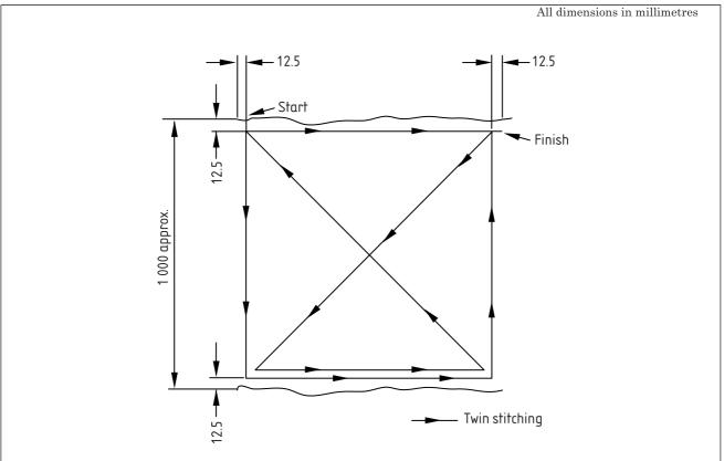
Figure A.1 — Test piece for threads of length per unit mass not less than 9 000 m/kg
