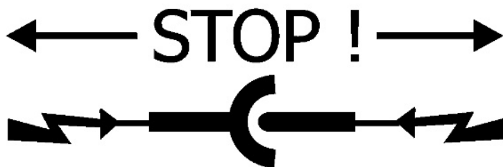
Figure A.1 – Symbol "DO NOT DISCONNECT UNDER LOAD"
